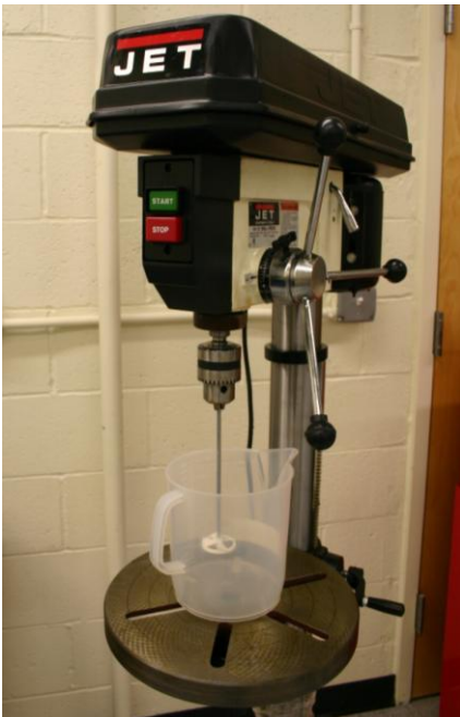
A variable speed drill press modified as mechanical mixer
