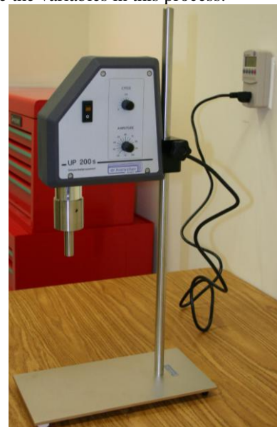
A sonotrode used in ultrasonic mixing.
