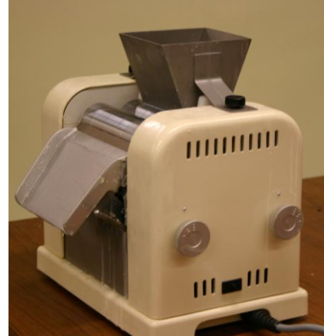
A three roll mill used for shear mixing.
