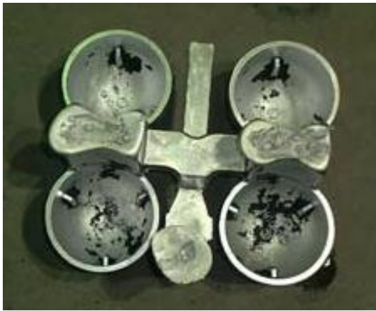
Figure 10. Four post cap casting made from Aluminum 319-10 vol% fly ash melt with gating.
