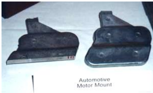
Figure 11. Automotive motor mounts of Al-fly ash made by squeeze casting.
