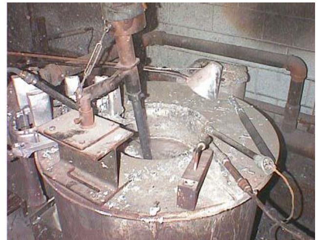
Figure 5. Typical melting and stirring setup for manufacturing aluminum matrix composites
